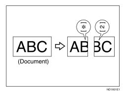
For example, this function splits the document if the document length is 20 mm (0.79") or longer than the paper used. The document is reduced if it is less than 20 mm (0.79"). When a document is split, an asterisk  $(\frac{\bigstar}{})$  is inserted at the split position and about 10 mm (0.39") of the split area is duplicated on the top of the second sheet.
